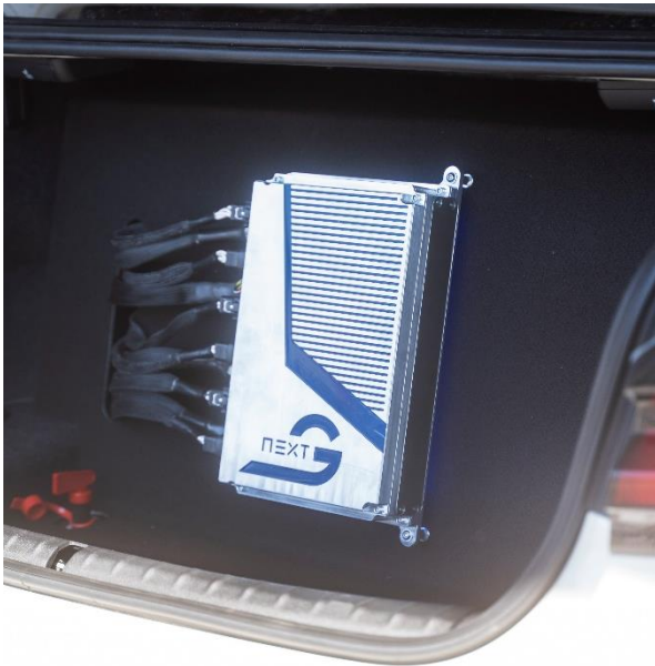
The central control unit in the test vehicle
