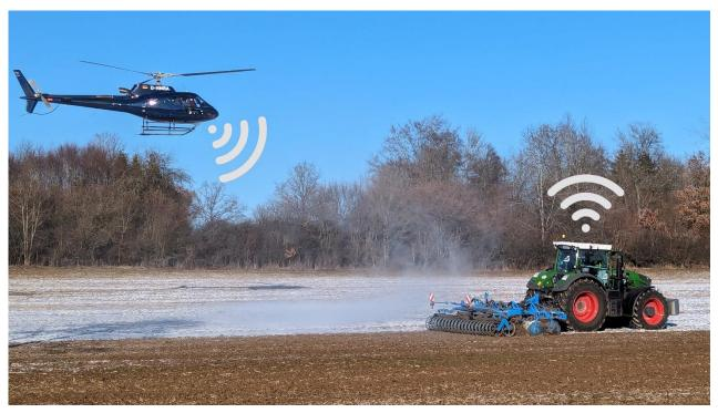
This tractor has been equipped with a redundant electronic steering and driving system from Arnold NextG and can therefore be teleoperated or driven remotely - even from a helicopter. Source: Arnold NextG I
