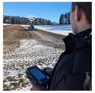
The digitalization of previously manual or hydraulic vehicle functions makes it possible to operate agricultural machines by remote control - without a human driver in the cab.
